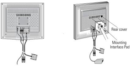
**1** Align the Mounting Interface Pad with the holes in the Rear Cover and secure it with the four screws that came with the Arm-type Stand or Wall Mount Hanger.
